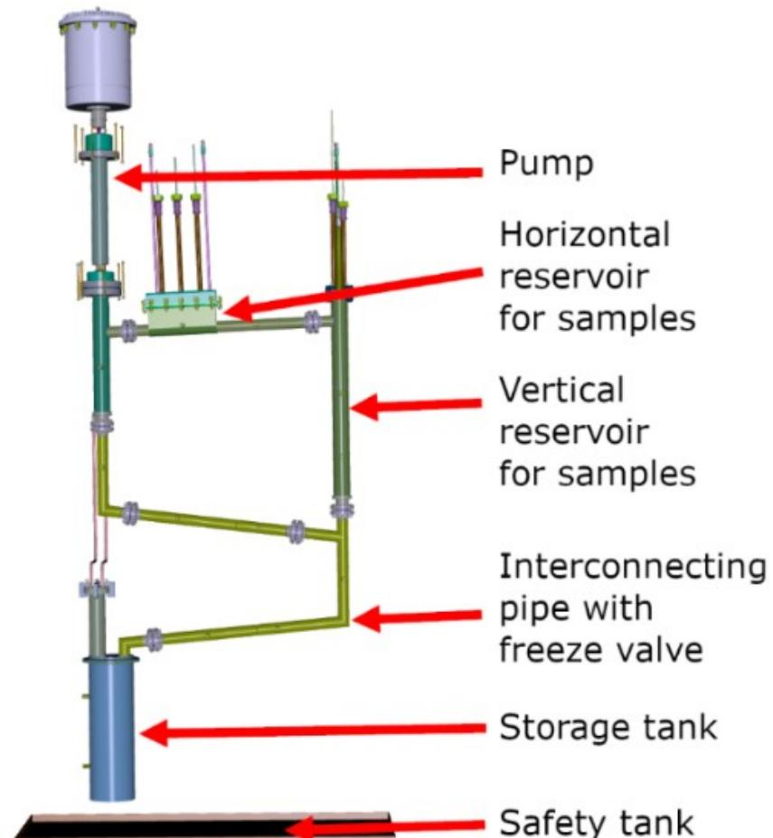
**Figure 2: Diagram of experimental loop MSL.**
