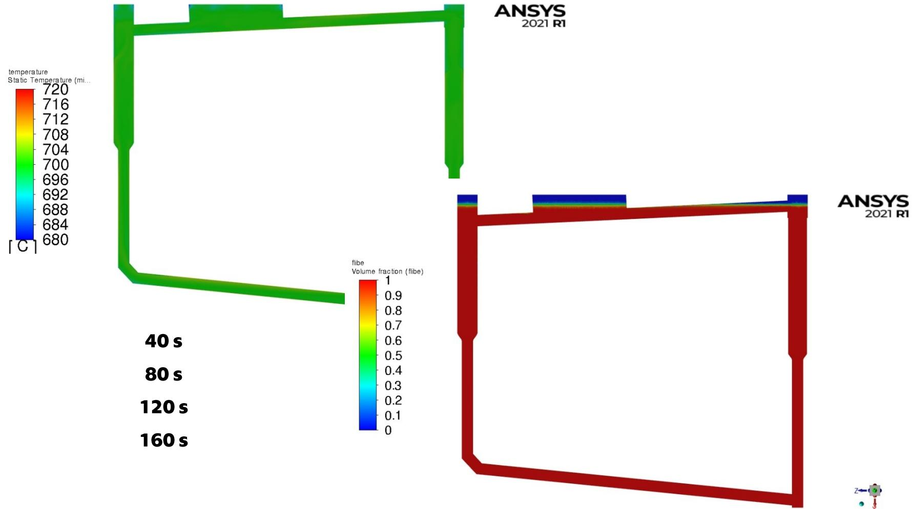
**Figure 7: Temperature field in cross-sectional symmetry during loop startup.**
