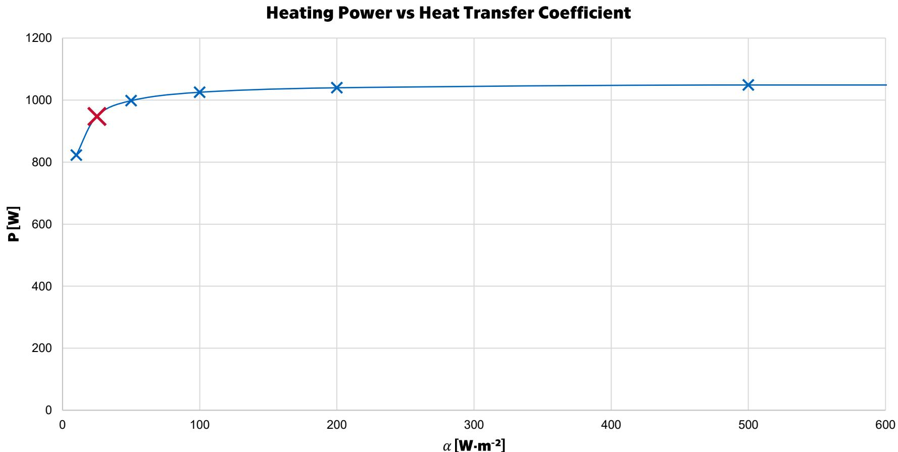
**Figure 4: Heating power dependency on the heat transfer coefficient between insulation and air.**
