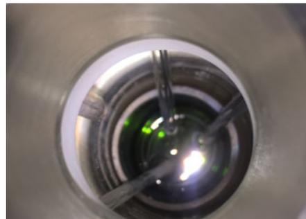
FLiNaK molten salt containing UF<sub>4</sub>
