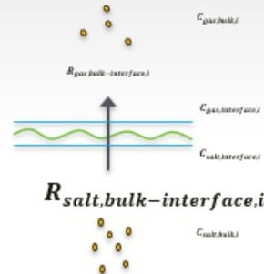
$$\frac{d(m_{i,j})}{dt} = kA(c_{gas,interface,i} - c_{gas,bulk,i})$$
