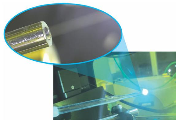
The plasma light is collected with a gated spectrometer to measure an elemental signature
